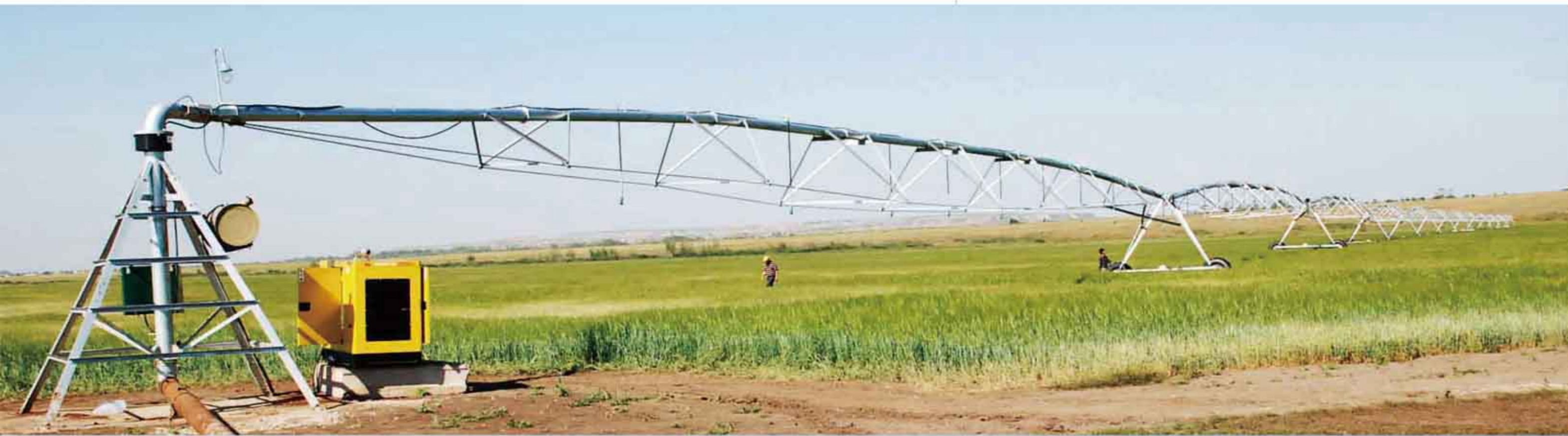
Rainfine 12 spans (650m) plus end gun with 12kw generator set in Kazakhstan 2011
